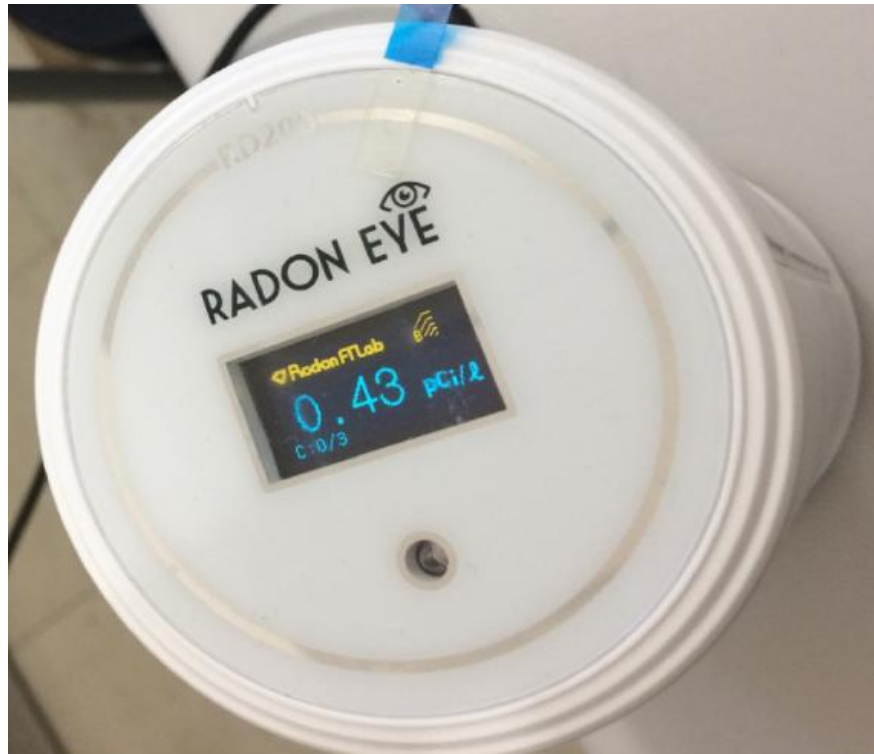
Fig. 1 – Top view of the RD200 RadonEye ionization chamber used to monitor radon gas
